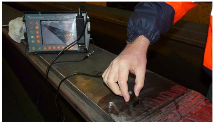
Non destructive testing on welded details
