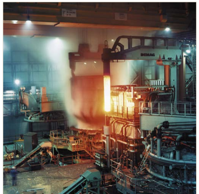
Electric arc furnace
