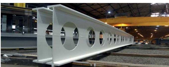
Final coating on fabricated girders
